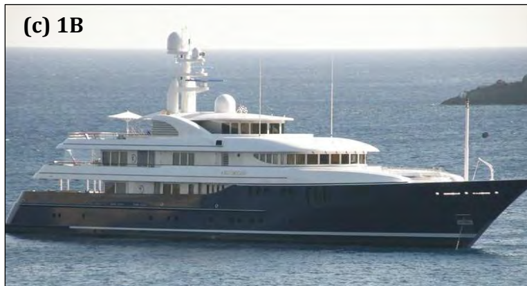
Figure 3. Examples of a: (a) Highly ice strengthened ship (CCGS Amundsen; Polar Class 3); (b) Medium ice strengthened ship (Acadia Desgagnés; Polar Class 7); (c) Little ice strengthened ship (Archimedes; Ice Class 1B). See Reference Box and Table 3 for further details.
